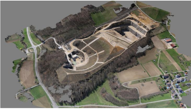
Figure 7. Automatically generated DSM (digital surface model) of an open pit mine with draped ortho-photo created from ca. 300 images taken with the SUSI 62
