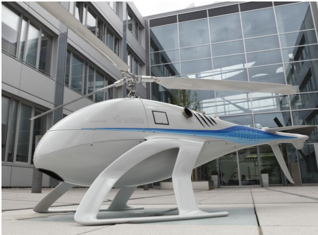
Fig. 1 Unmanned Mission Avionics Test Helicopter based on Swiss UAV NEO S-350 Twin
