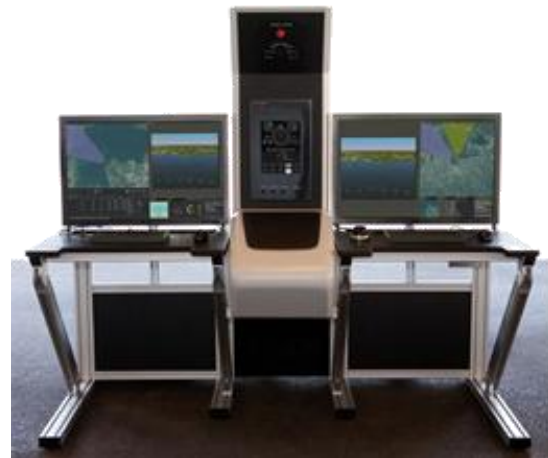
Fig. 2 Current Ground Control Station of the Swiss UAV NEO S-350 Twin
