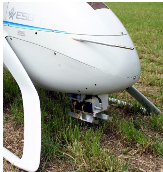
Fig. 11 SAR sensor package mounted on UMAT
