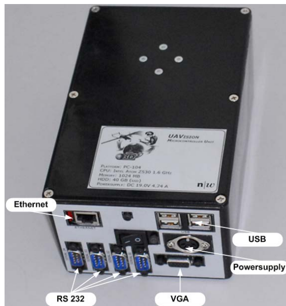
Figure 3: UAVision payload controller in custom casing with the different interconnects
