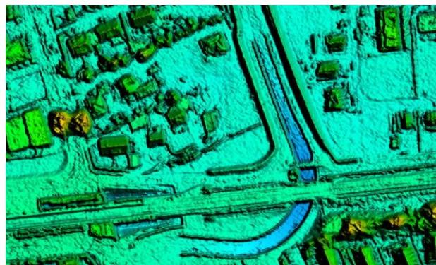
Figure 8 DSM section, road under-passing the train tracks
