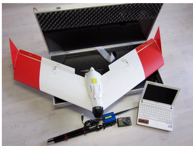
Figure 2 PAMS' SmartOne UAV with transport box, groundstation computer, accessories
