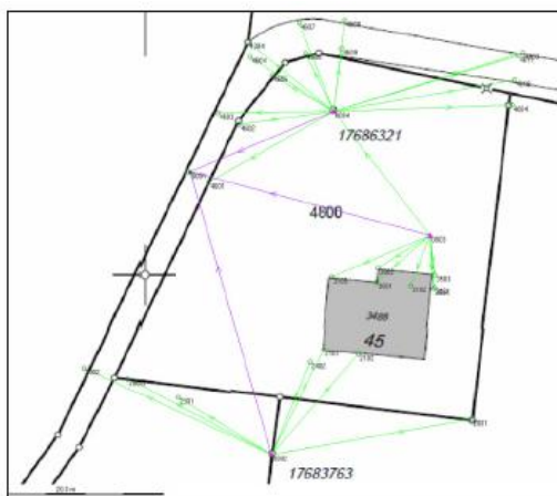
Figure 4. Site map from the Swiss official cadastral surveying including the achieved measurements using tachymetry/GNSS (test site Krattigen)
