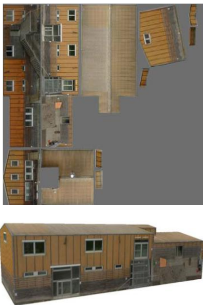
Figure 12. Texture components and the 3D-Model derived from UAV images of the HXE-building at Campus Science City Campus ETH Hoenggerberg, displayed in VRMLVIEW
