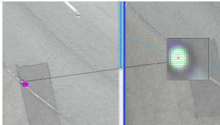
Figure 9. Determination of the target centre points using the centroid operator
