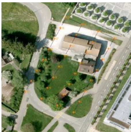
Figure 2. Flight planning of the test area Campus Science City ETH Hoengerberg
