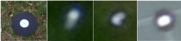
Figure 8. The original target (left) and the corresponding targets in the image with motion blur
