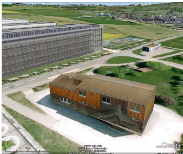
Figure 13. 3D-Model derived from UAV images of the HXE-building at Campus Science City ETH Hoenggerberg, imported to Google Earth
