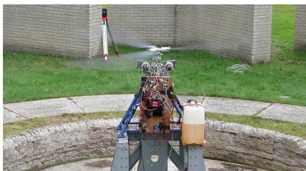
Figure 8. Endurance Test of Geocopter GC-201
