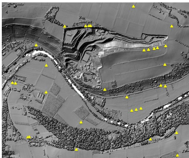
Figure 4: Test-site Vaihingen/Enz, with signalized points overlaid to shaded DSM from airborne LiDAR
