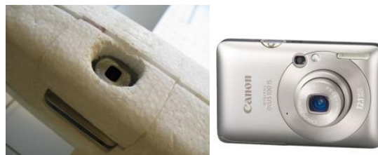
Figure 3: Used consumer camera and mounting position on UAV belly
