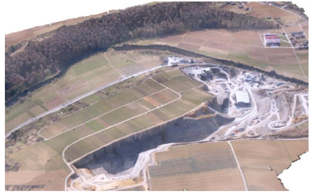
Figure 11: Perspective view of UAV ortho image draped over computed DSM
