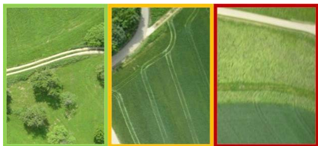
Figure 5: Three images patches with sharpness values. Left: low image blur (0.18, green), middle: moderate image blur (0.36 yellow) and high image blur (0.38, red).
