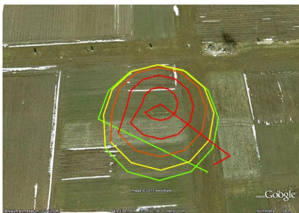
Figure 1: Flight pattern for BRDF-measurements
