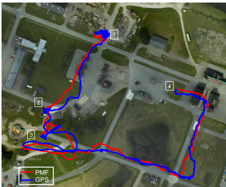
Figure 9: Real-time on-board position estimation results. Comparison between the flight path computed with the PMF (red) and the GPS reference (blue).
